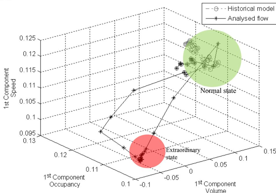
**Fig 5.** Traffic state vectors in the new reduced dimension. The figure compares two-hour flows from the example shown above, but with common component dimension. Grey dashed plots represent historical model from equivalent day and time period. Black plots represent flow with detected incident. We see that incident values lies out of model cluster and can be identified based on distance from the model state in discrete time
