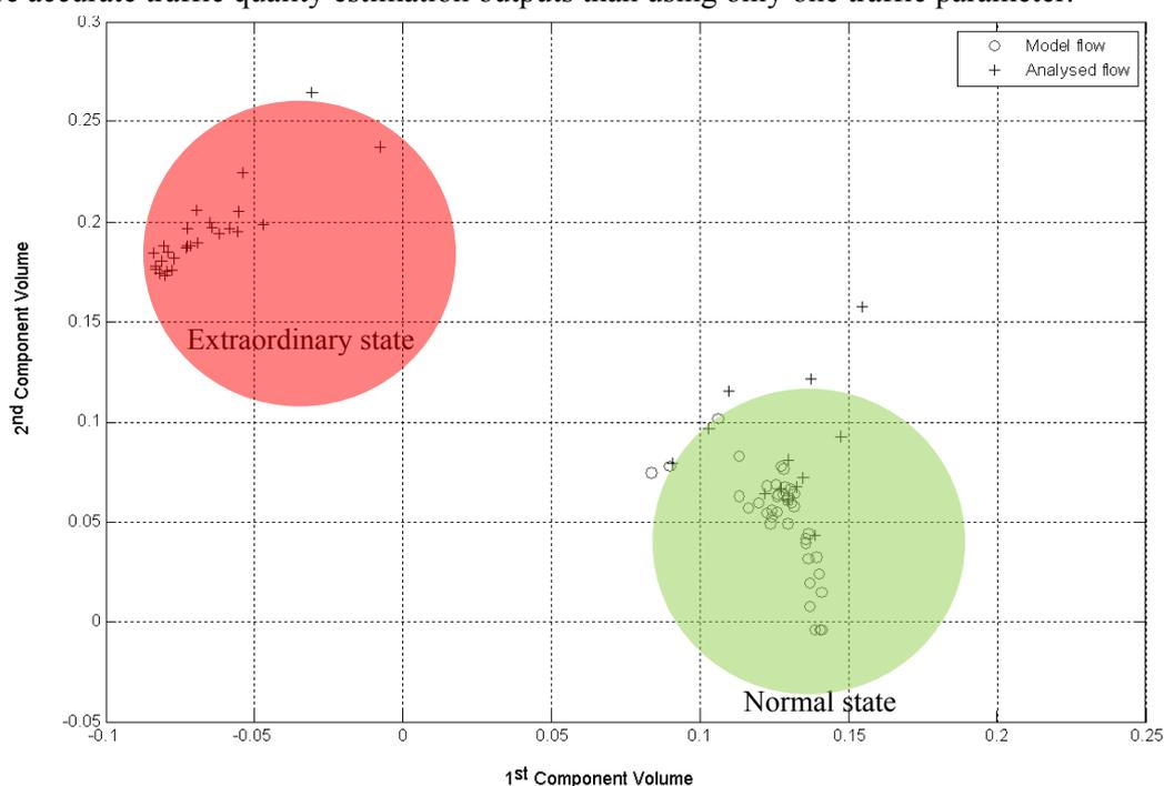
**Fig 4.** First and second PC coordinates of normal vs. extraordinary traffic situation based only on volume data projected into new dimension
