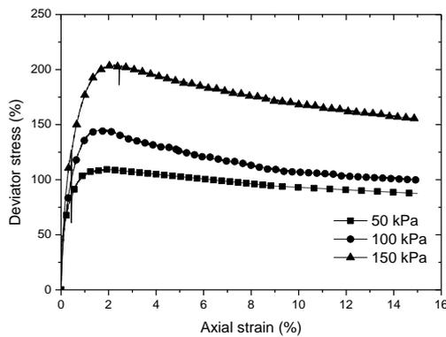
Figure 4. Stress-strain curves for large samples
