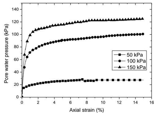
Figure 5. Pore pressure results versus axial strain for large triaxial test
