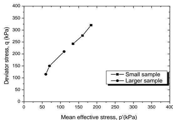
Figure 6. Peak strength envelopes of small samples and large samples
