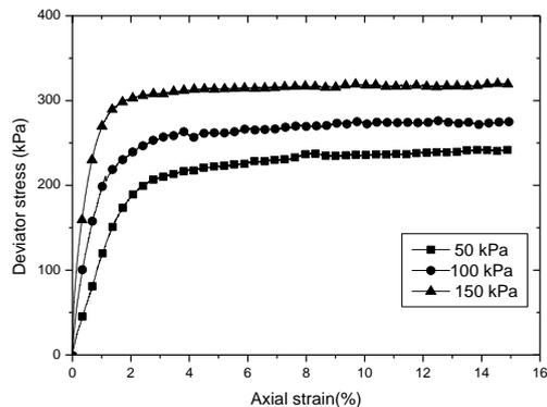
**Figure 2.** Stress-strain curves for small samples
