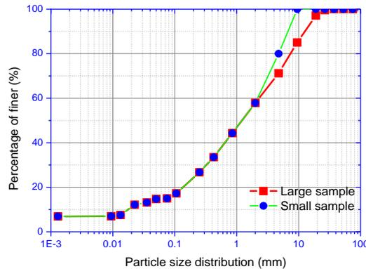
Figure 1. Particle size distribution of waste mixture samples for small and large triaxial tests
