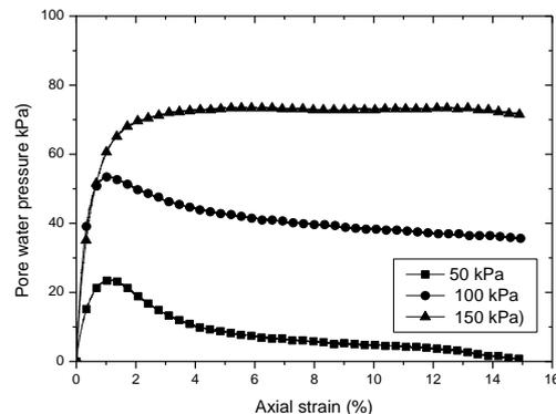
**Figure 3.** Pore pressure results versus axial strain for small triaxial test
