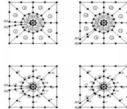
Figure 20. Element technique of simulating a crack tip
