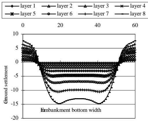
Figure 7. Consolidation process during embankment fill
