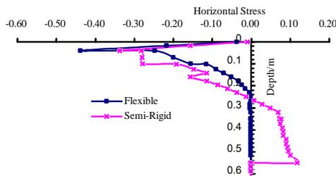
Figure 14. Horizontal stress at deflection point
