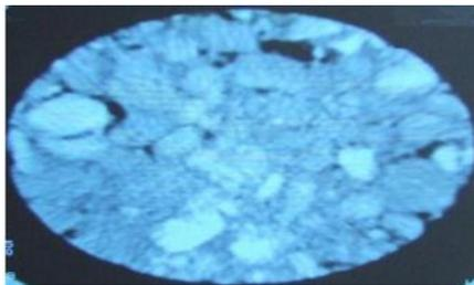
**Figure 24.** CT scanned AC specimen
