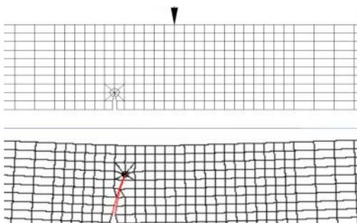
Figure 19. Crack propagation of testing
