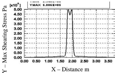
Figure 18. Shearing stress of rectangular loading
