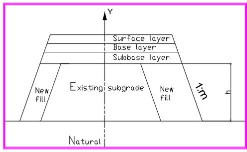
Figure 11. Pavement over road-widening section
