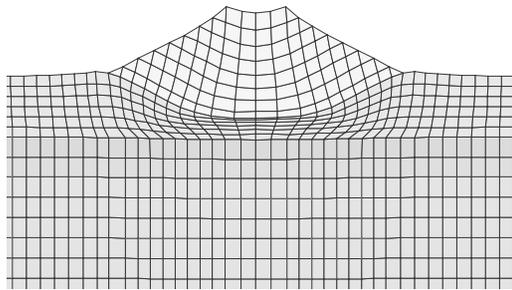
**Figure 5.** *Deformation characteristics of flat ground*
