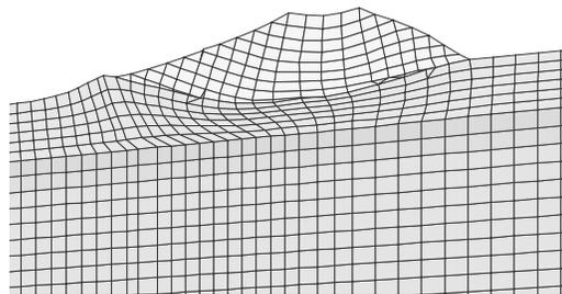
**Figure 6.** *Deformation characteristics of sloped ground*
