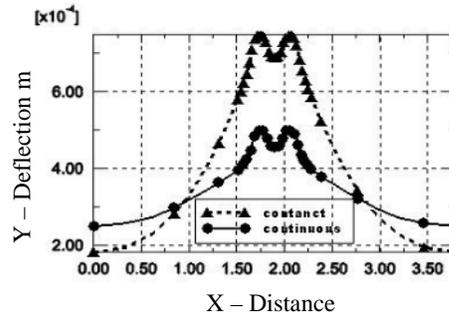
Figure 15. AC pavement surface deflection
