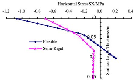
Figure 13. Maximum horizontal stress of AC layer
