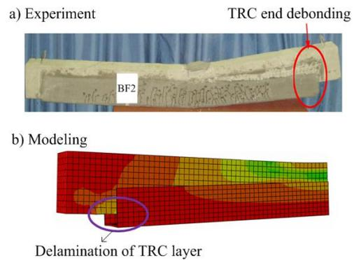
**Figure 8.** Failure mode of strengthened beam BF2
