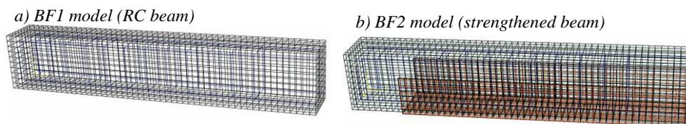
Figure 4. Mesh for ABAQUS models
