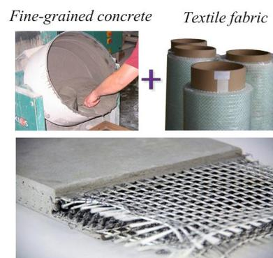
**Figure 1.** Textile reinforced concrete
