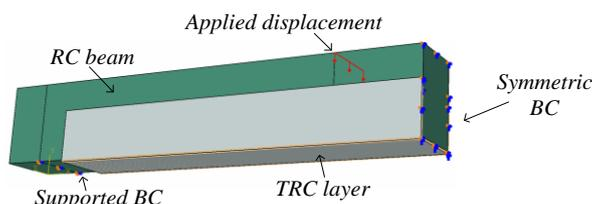
Figure 3. FE model of RC beam strengthened with TRC layer
