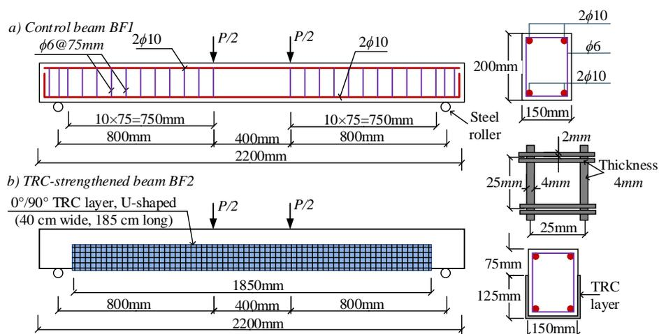
**Figure 2.** Details of beam specimens [2]
