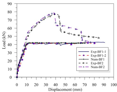
**Figure 7.** Load-displacement curves of BF1 and BF2 beams
