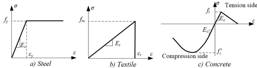
Figure 5. The stress-strain relationship for the steel, textile, and concrete materials
