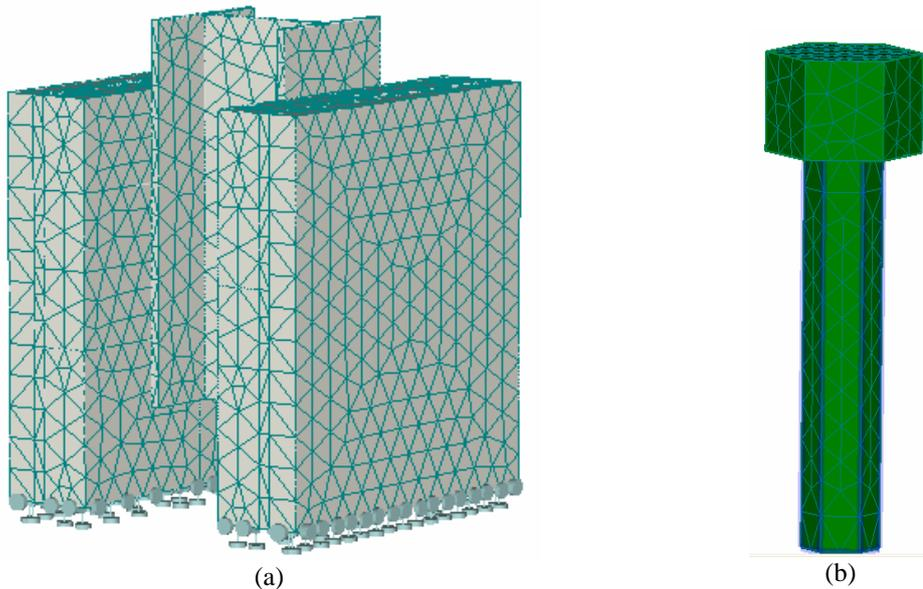
**Figure 4.** Finite element mesh: a) slab concrete and steel beam ; b) stud
