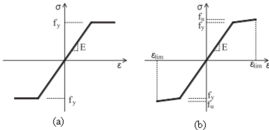
**Figure 3.** Stress-strain for: (a) steel of stud and beam; (b) reinforcement
