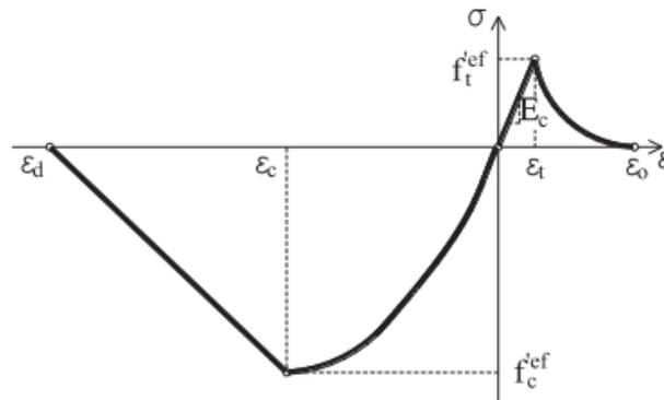
**Figure 2.** Stress-strain law for concrete
