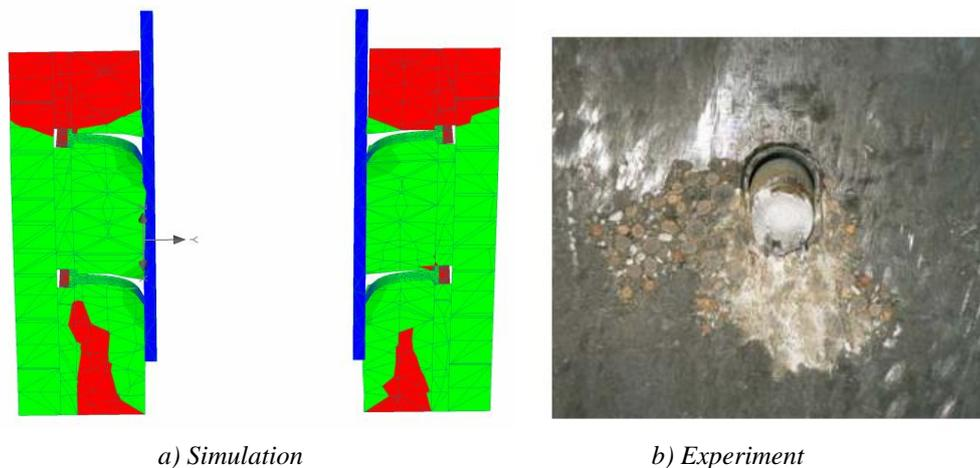
**Figure 5.** Deformed shapes of studs
