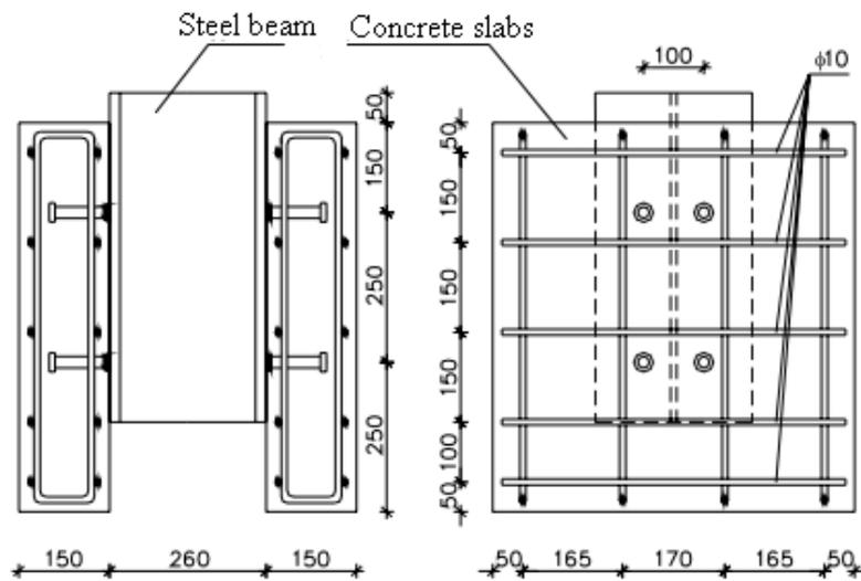
Figure 1. Push-out test specimen
