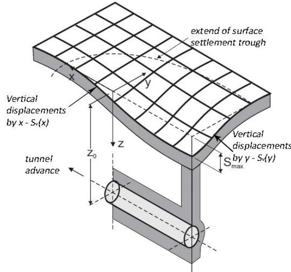
**Figure 5.** Character of the ground surface settlements under tunnel construction:  $y$  – the transverse direction;  $x$  – the longitudinal direction (along the tunnel centerline)
