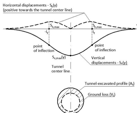
**Figure 6.** The horizontal and vertical displacements of the ground surface at the transverse direction of the tunnel center line
