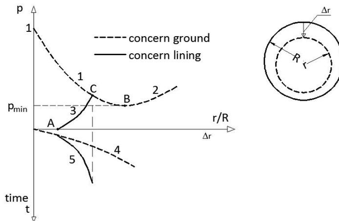
**Figure 3.** The interaction between the ground and the support (sprayed concrete lining): 1 – ground response curve; 2 – loosening curve; 3 – the support response curve; 4, 5 – dependence of the displacement of tunnel-excavated profile on time respectively in the case of absence and presence of the support.  $p_0$  – initial effective ground pressure on the tunnel-excavated profile (radius  $R$ ) and  $p$  – effective ground pressure on the tunnel-excavated profile with the radius  $r$
