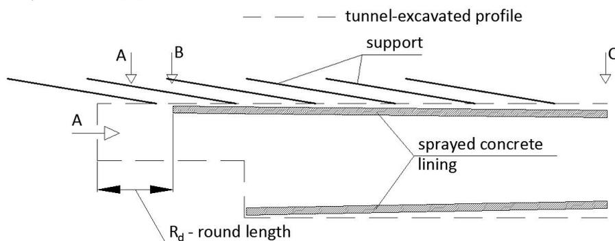
**Figure 4.** Main components of ground deformations around the tunnel-excavated profile: A – ground movement towards unsupported heading, B – radial ground movement towards the lining and C – radial ground movement towards the lining due to consolidation.
