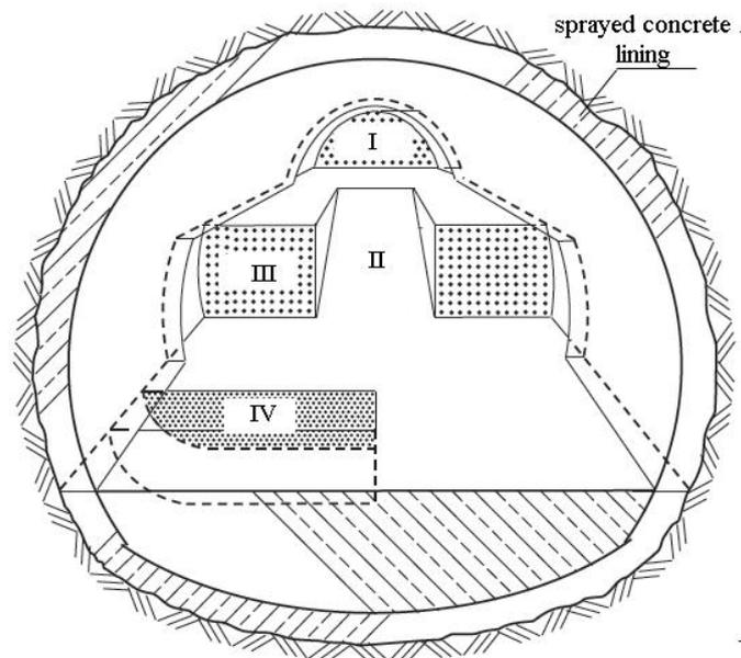
**Figure 1.** Sequence of the excavation in tunnel construction by applying NATM technologies: I – crown excavation; II – center bench excavation; III – lateral bench excavation; IV – invert excavation
