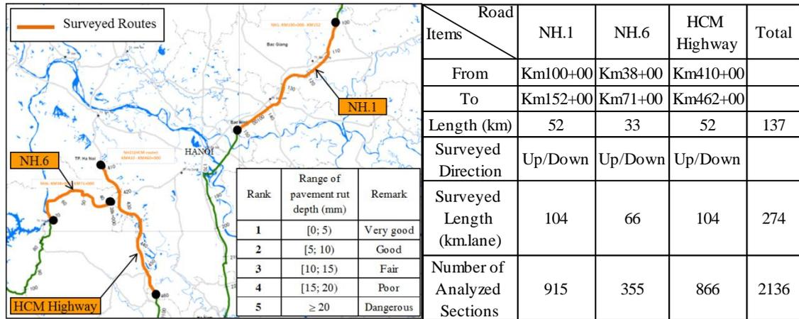
**Figure 2.** Location and information of selected highways for pavement condition surveying and definition of ranking for pavement condition in rutting
