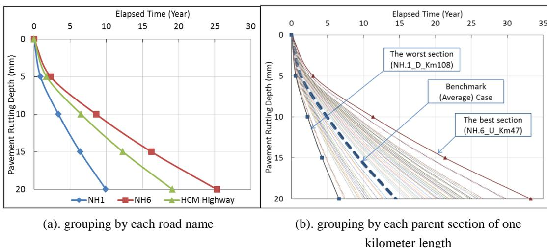
**Figure 3.** Pavement rutting deterioration curves estimated by Local Mixture Markov Hazard Model
