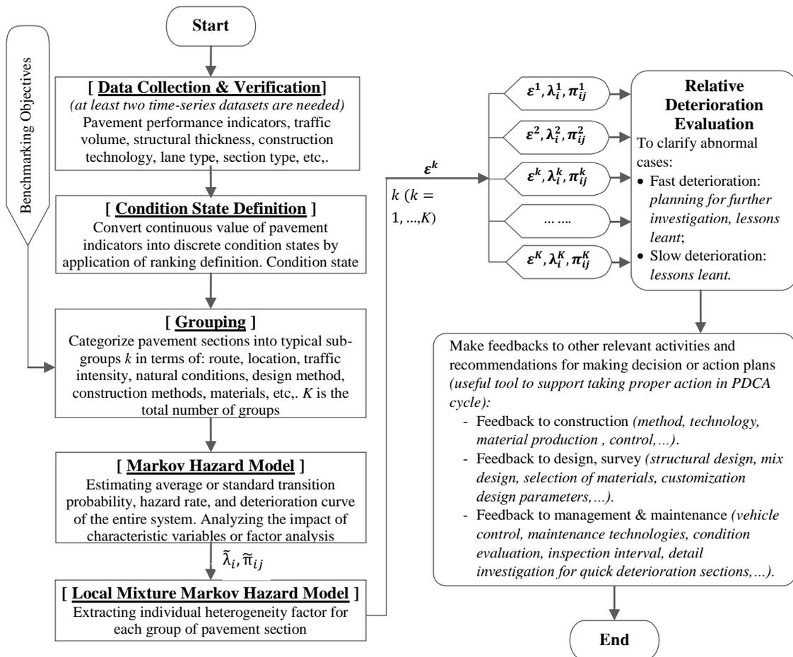
Figure 1. Flowchart to evaluate pavement deterioration by the Local Mixture Markov Hazard Model
