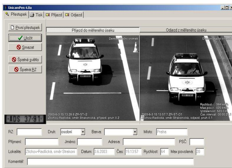
*Fig 2. Photo at entry of measured section (left) and the same car at exit (right).
