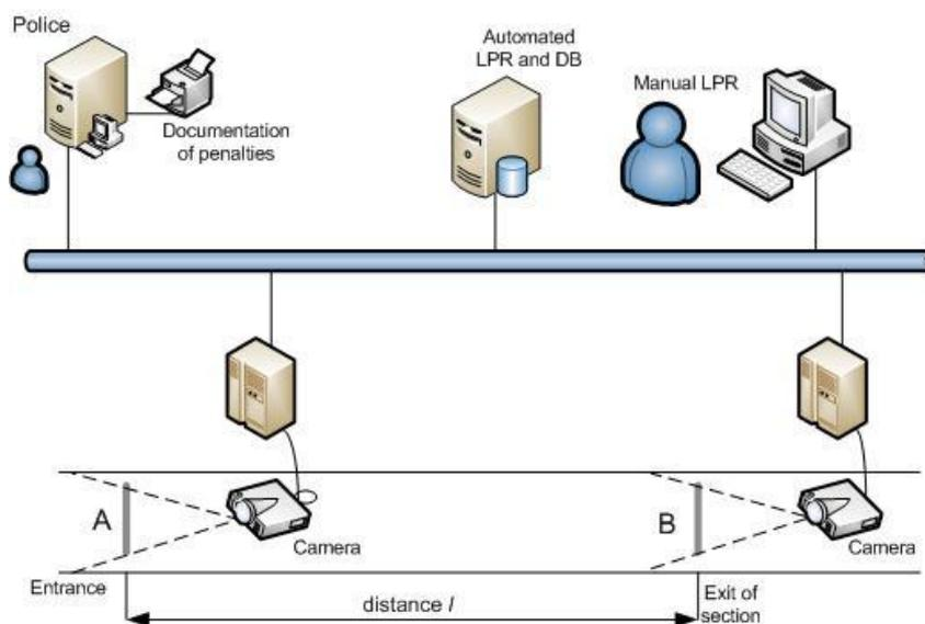
*Fig 1. Principal scheme of Section Speed Control*
