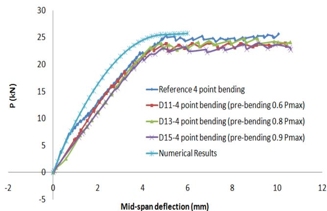
**Figure 7.** Load versus mid-span deflection of tested beams in 3PB (4PB pre-loaded)
