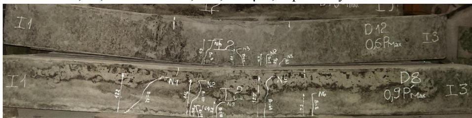
**Figure 6.** Cracks in RC beam preloaded in 4PB test ( $P = 0.6P_{max}$  and  $P = 0.9 P_{max}$ )
