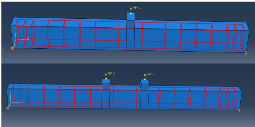
**Figure 5.** Model of concrete beam in 3PB and 4PB test
