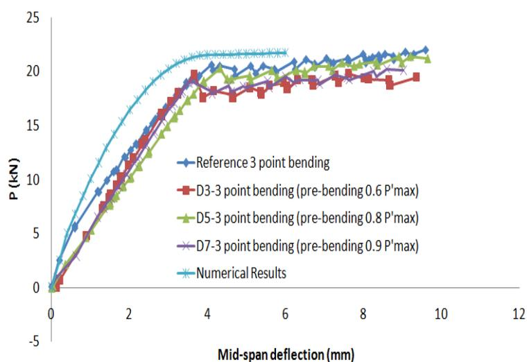
**Figure 8.** Load versus mid-span deflection of tested beams in 4PB (3PB pre-loaded)
