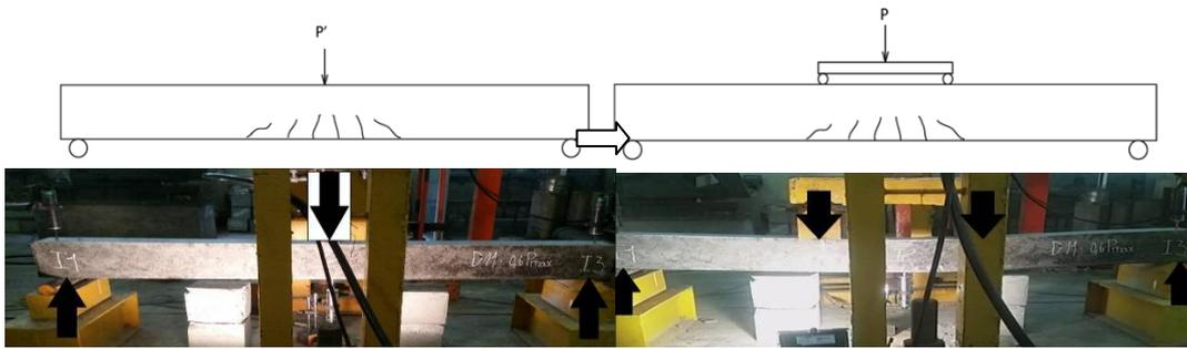
**Figure 4.** 4PB test of cracked beams after preloaded in 3PB test
