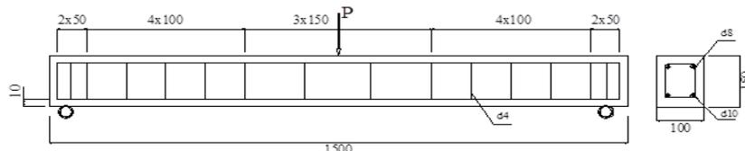
**Figure 1.** Beam specimens with reinforcement arrangement
