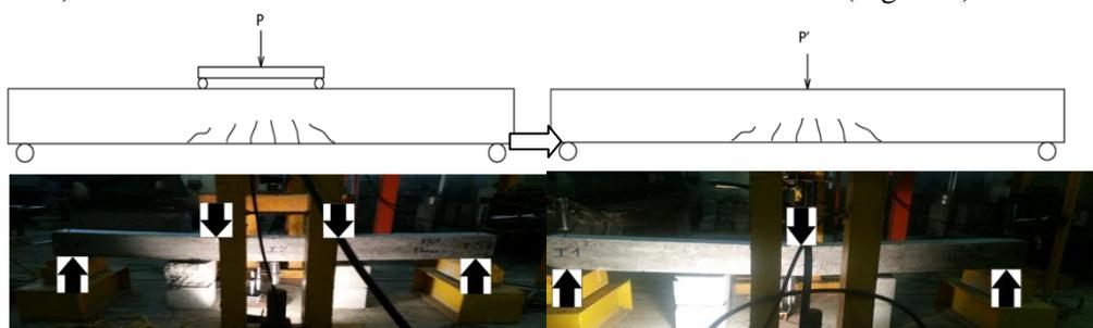
**Figure 3.** 3PB test of cracked beams after preloaded in 4PB test
