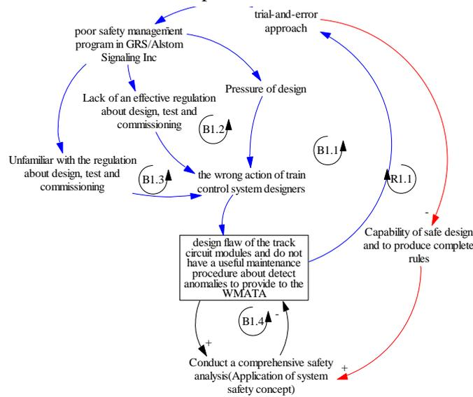
Fig 5. Causal loop diagram for the collision Accident about design flaw
