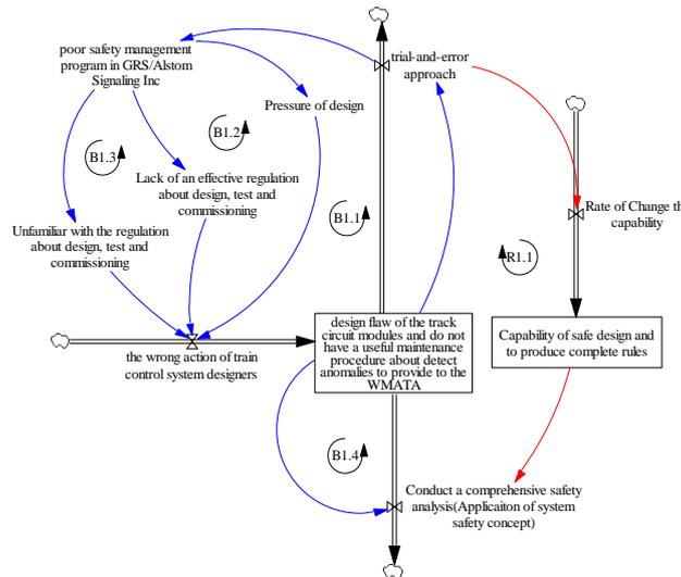
**Fig 6.** The stock and flow diagram of design flaw of the track circuit modules
