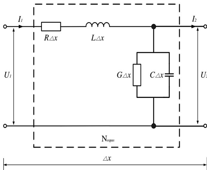
*Fig 1. Schematic diagram of transmission line equivalent four-port network*
