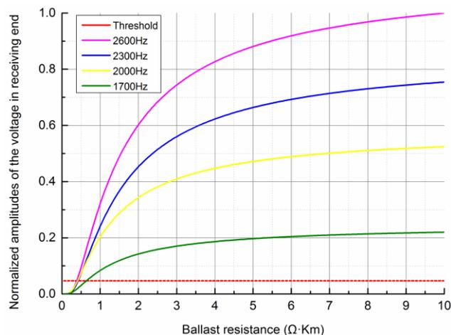
**Fig 5.** Influence of ballast resistance on the receiving-end voltage of track circuit
