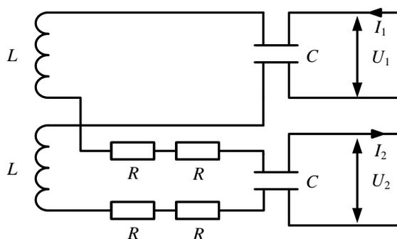
Fig 3. Structure diagram of 2 Km simulation cable
