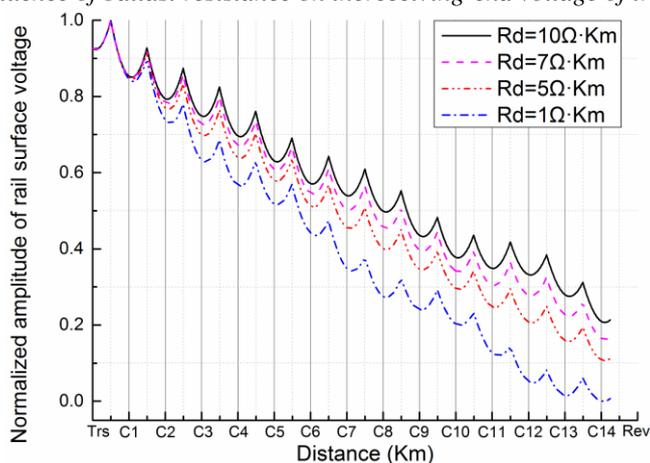
**Fig 6.** Influence of ballast resistance on rail surface voltage of track circuit
