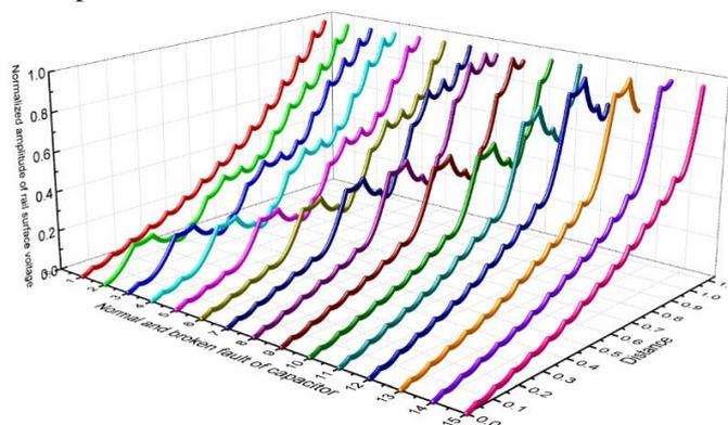
Fig 7. Influence of compensation capacitor failure on transmission characteristics of track circuit
