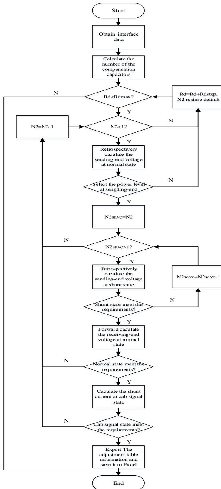
Fig 4. Establishment logic of the track circuit adjustment table
