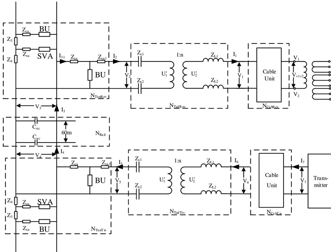
Fig 2. Schematic diagram of the jointless track circuit
