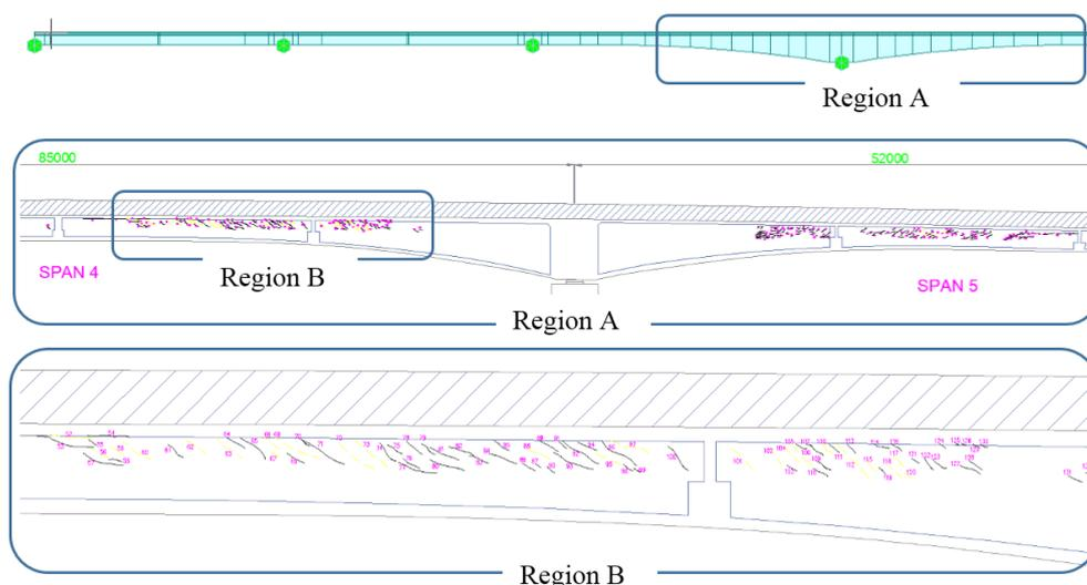
*Figure 1. Crack pattern in the inside of the box girder of bridge*
