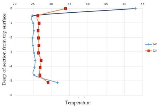
**Figure 7.** Thermal gradient on the height of web (vertical direction)
