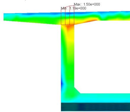
**Figure 10.** Distribution of thermal principal stress 1 in in the width of web (horizontal direction)
