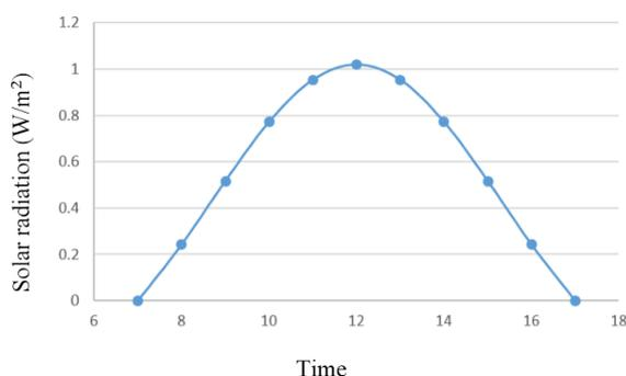
**Figure 3.** Daily change of solar radiation on the bridge surface
