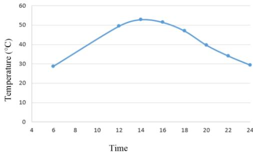
**Figure 5.** Daily distribution of temperature on the top surface
