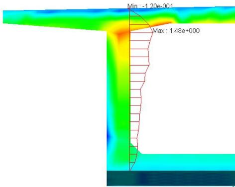
**Figure 9.** Distribution of thermal principal stress 1 in in the height of web (vertical direction)
