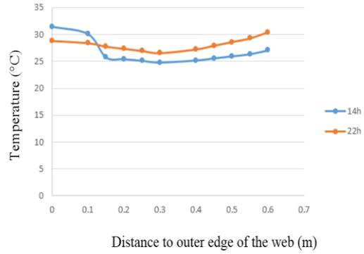
**Figure 8.** Thermal gradient on the width of web (horizontal direction)
