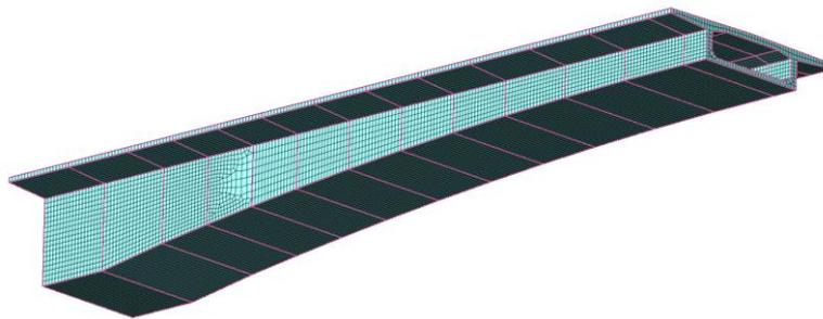
*Figure 2. Finite element model for the bridge girder*
