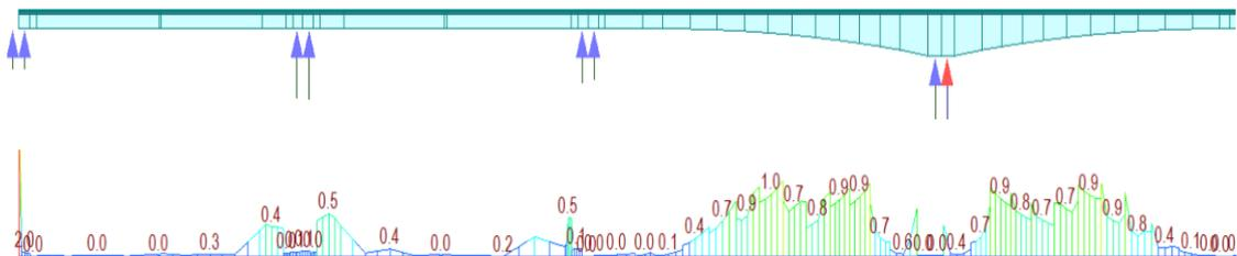
**Figure 11.** Distribution of principal stress 1 caused by dead load and prestress on the beam length
