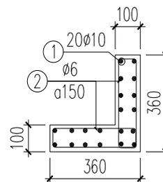
Figure 3. Section design of test specimen
