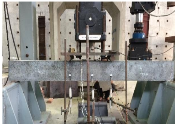
Figure 6. Flexural test setup for beams
