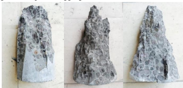
Figure 3. Destructive form of LWAC axial compressed test
