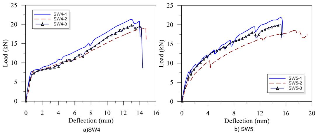
**Figure 4.** Load – deflection results of specimen SW4 and SW5
