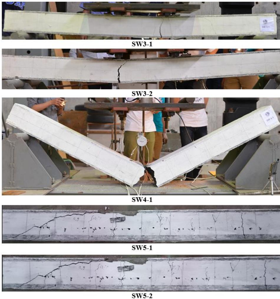
**Figure 6.** Crack pattern of tested sandwich beams
