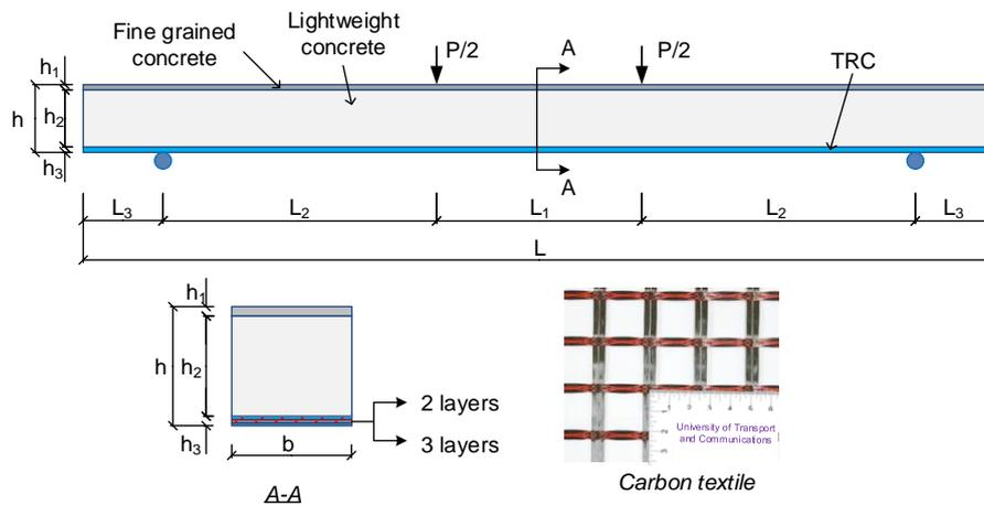
Figure 1. Test specimens
