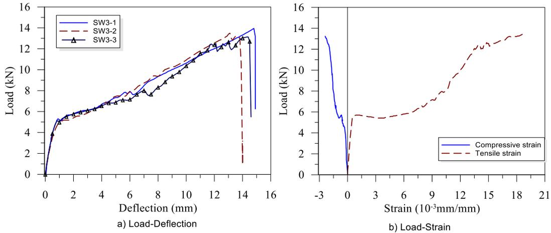
**Figure 3.** Experimental results of sandwich panel SW3
