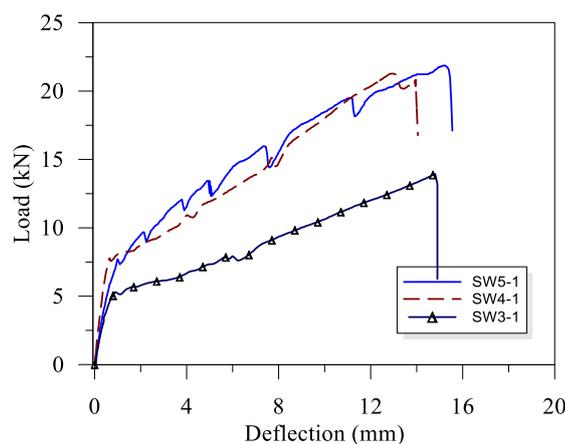
**Figure 5.** Comparison of load and deflection between specimens SW3-1, SW4-1 and SW5-1
