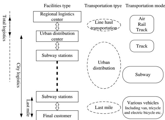
Figure 6. Basic composition of vehicle-subway urban distribution
