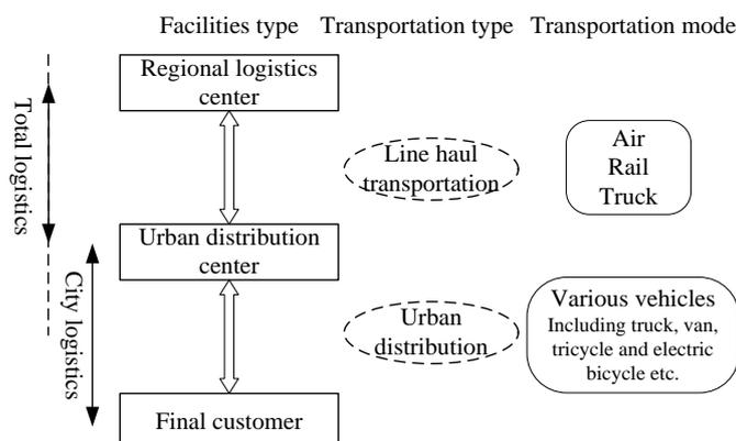
*Figure 1. The basic structure of existing urban distribution network*
