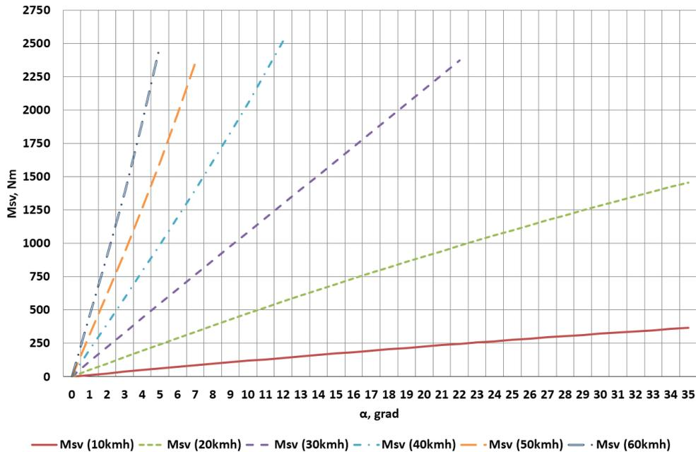
Fig 4. Dependence of speed stabilization moment on wheels rotation angle
