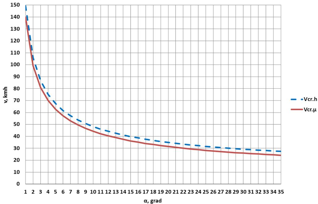
Fig 3. Dependence of critical speed on wheels rotation angle
