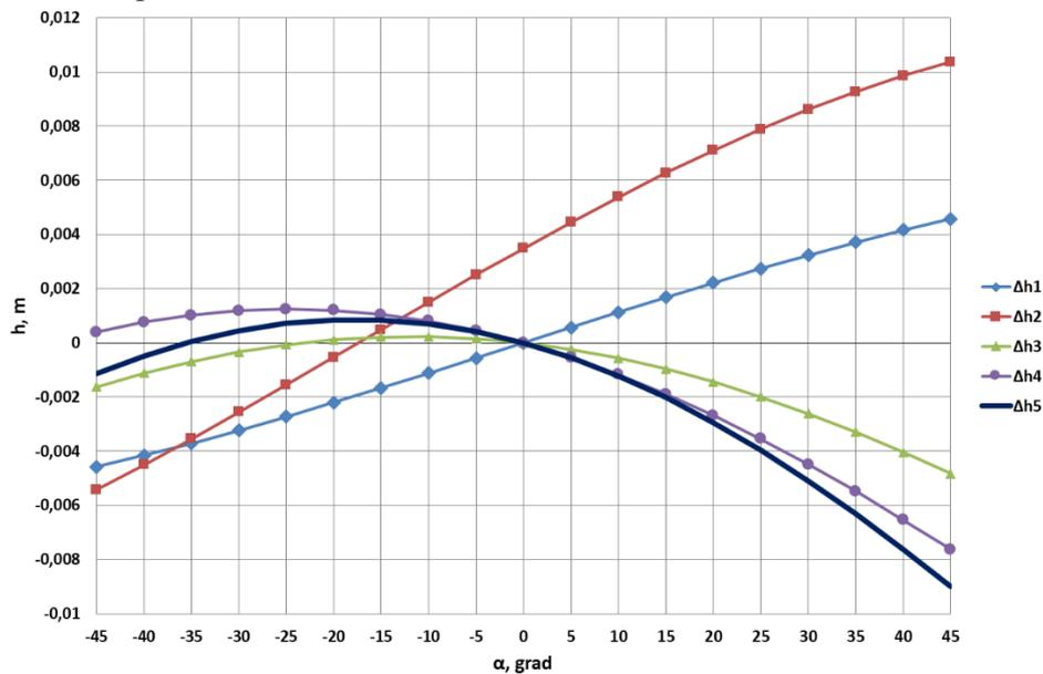
Fig 6. Dependence of the body lift height on wheel rotation angle
