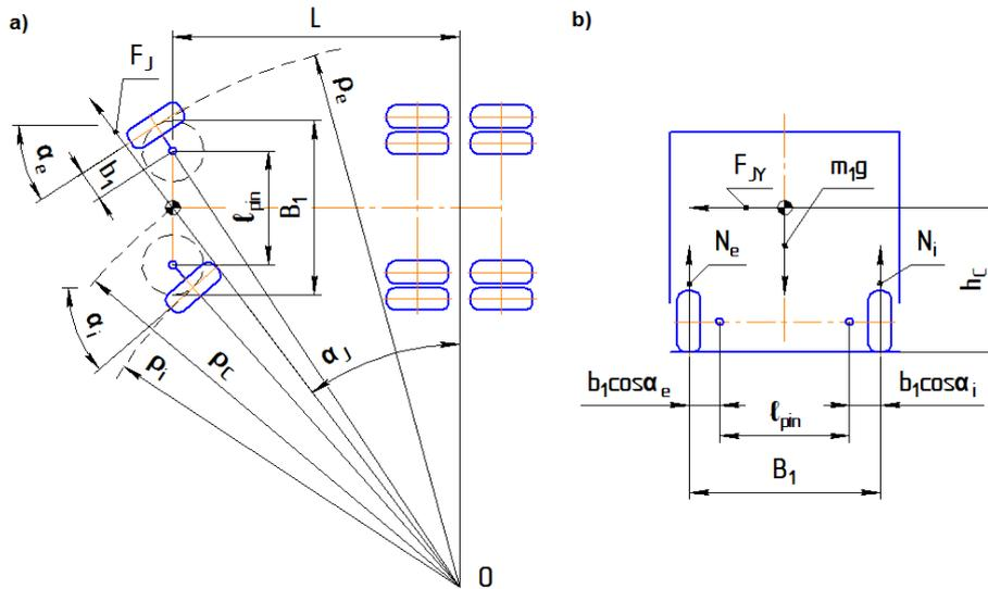
Fig 2. Kinematic (a) and force (b) rotation patterns
