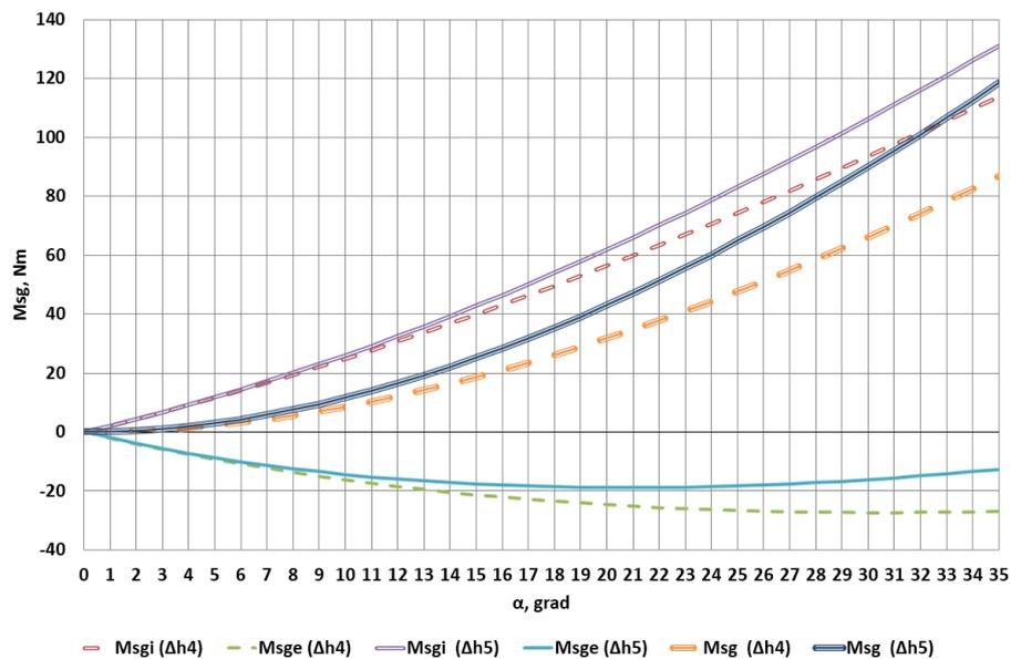
Fig 7. Dependence of weight stabilization moment on wheels rotation angles
