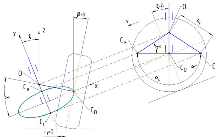
**Fig 5.** Influence of the kingpin lateral inclination on the trunnion trajectory
