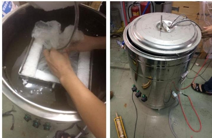
*Figure 2. Placing concrete sample in adiabatic calorimeter.*
