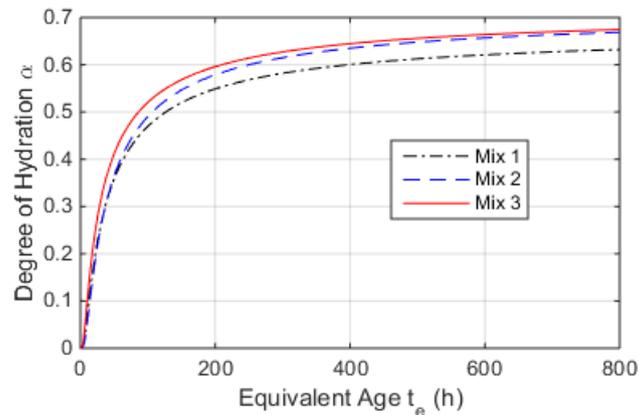
**Figure 5.** Degree of hydration curves for 3 concrete mixes.
