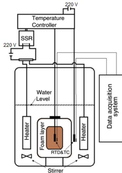
*Figure 1. Schematic diagram of adiabatic calorimeter (Lin and Chen, 2015)*
