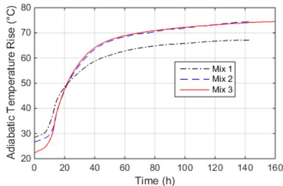
**Figure 3.** Measured ATR for mixes.
