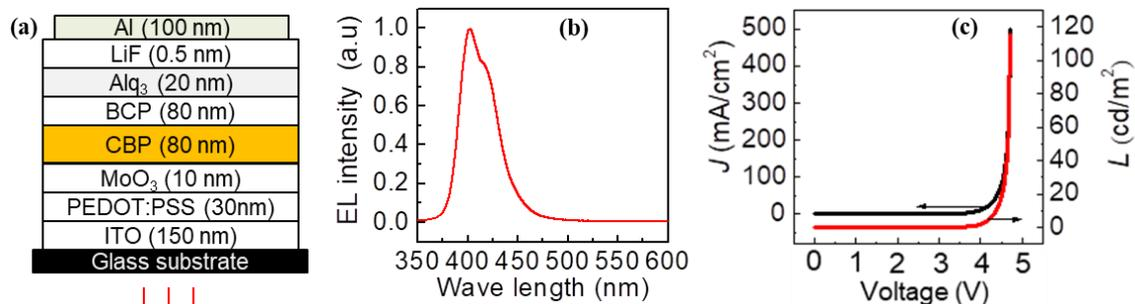
**Figure 2.** a, OLED device structure. c, EL spectra. d, J-V-L relationship of OLED.
