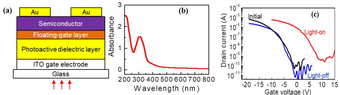
**Figure 3.** a, PhotoOTFT device configuration. b, Absorbance spectra of gate dielectric layer. c, Electrical characteristics corresponding to changes in the light at voltage of 5 V.
