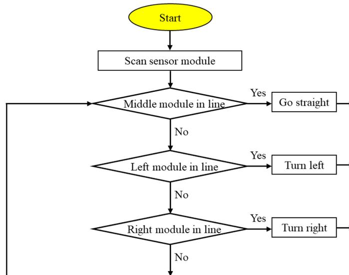
**Figure 8.** Flowchart for control functionality using UV photosensor.
