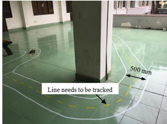
**Figure 6.** Test track circuit made in University laboratory.
