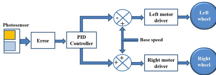
**Figure 7.** Diagram control for line tracking.
