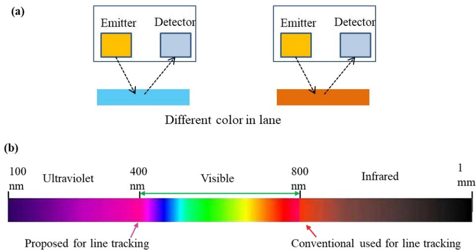
**Figure 1.** a, Line tracking principle based on photosensor. b, Illustration of light spectrum and a proposed UV light for line tracking.
