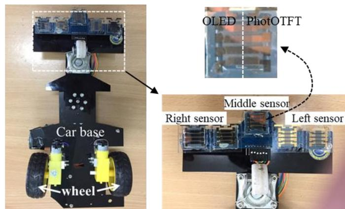
Figure 5. Photos of autor car with photosensor mounted on car, OLED and photoOTFT on substrate module
