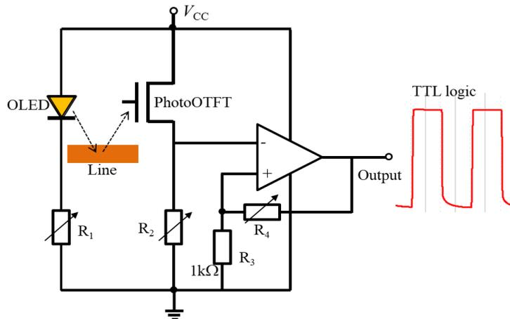
Figure 4. Encoder circuit module for photosensor.
