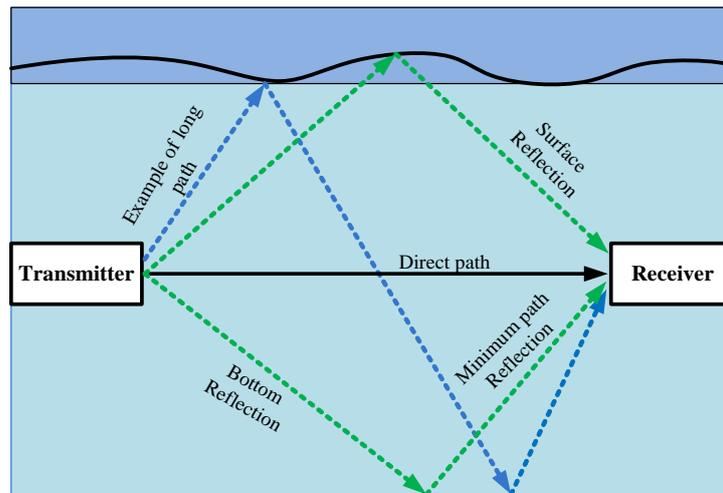
**Figure 2.** Diagram of simple multipath channel used in this MATLAB simulator [13]
