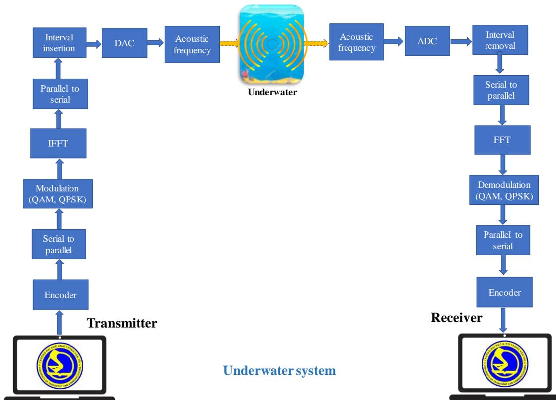
*Figure 1. Block diagram OFDM-based channel model in this simulation*
