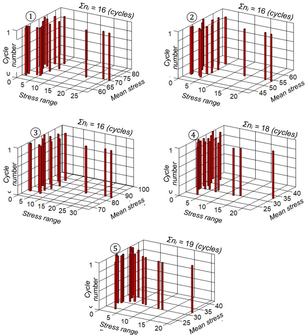
**Figure 9.** Statistical characteristics of hot spot stress-time histories with 150 load steps
