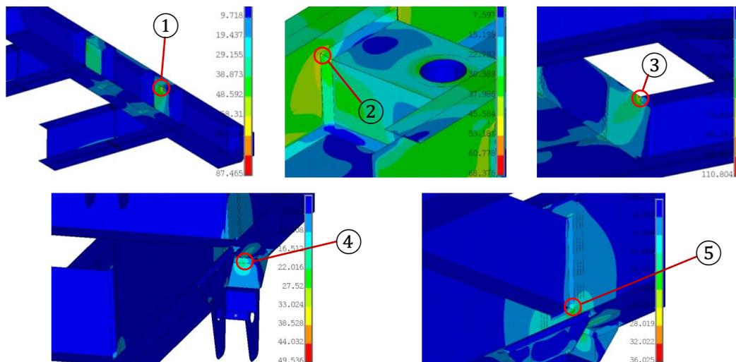
Figure 7. Equivalent stress distribution of typical critical locations
