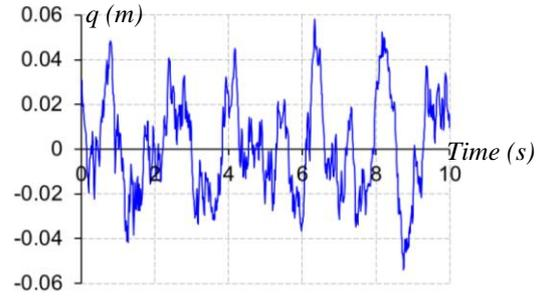
**Figure 5.** Road roughness of D grade with vehicle speed of 60 km/h.
