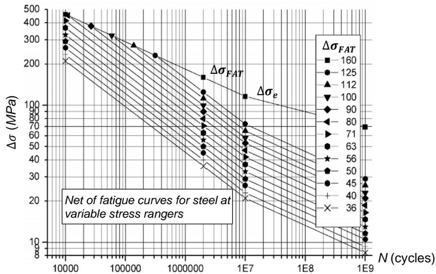
Figure 6. Fatigue curves correspond with the fatigue classes ( $\Delta\sigma_{FAT}$ )
