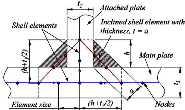
**Figure 2.** The modeling of fillet welded joint using inclined shell elements
