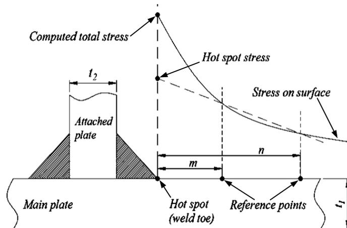
**Figure 1.** Sample surface extrapolation of the reference points to the weld toe in order to approximate the structural hot spot stress.
