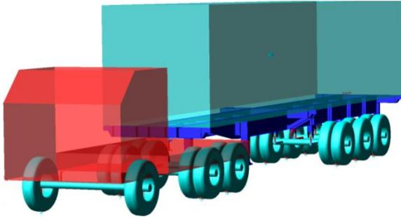
**Figure 4.** The MBD model of full vehicle in ADAMS software.
