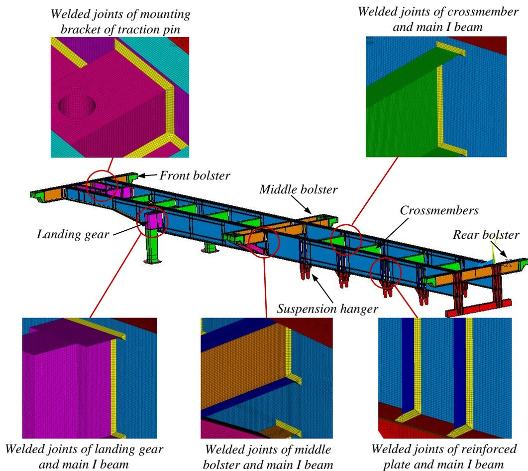
**Figure 3.** The FE model of chassis frame with some typical fillet welded joints
