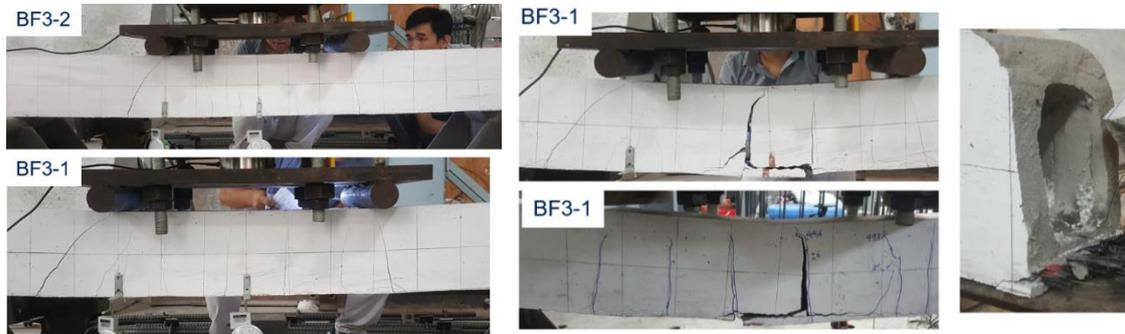
**Figure 9.** Crack patterns of long beams with 3 textile layers
