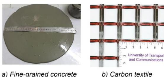
**Figure 3.** Carbon textile and fine-grained concrete
