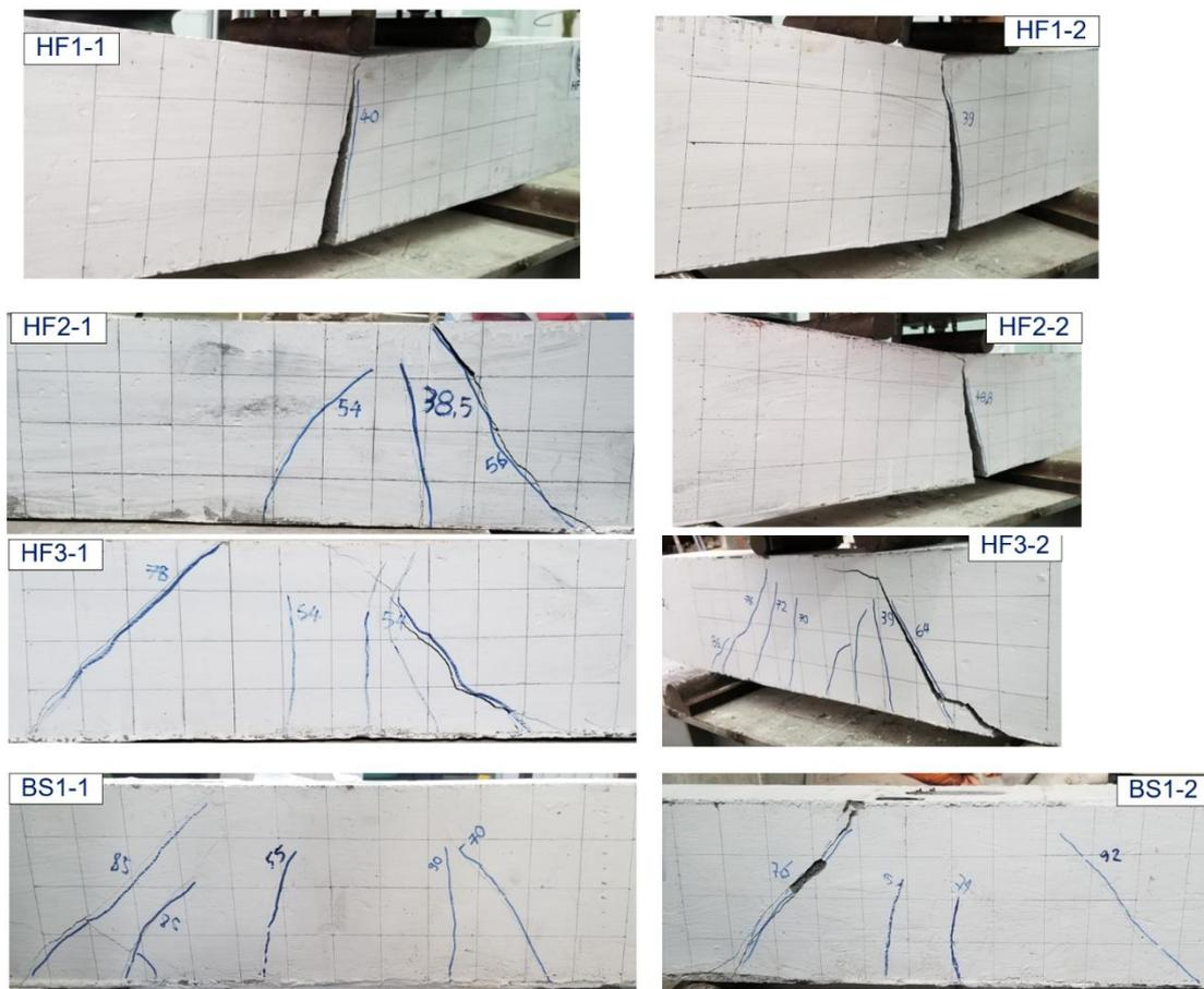
**Figure 7.** Crack patterns of short beams in 1<sup>st</sup> group
