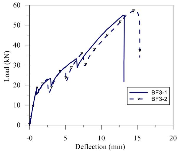
**Figure 8.** Load-deflection curves of two long beams in 2<sup>nd</sup> group
