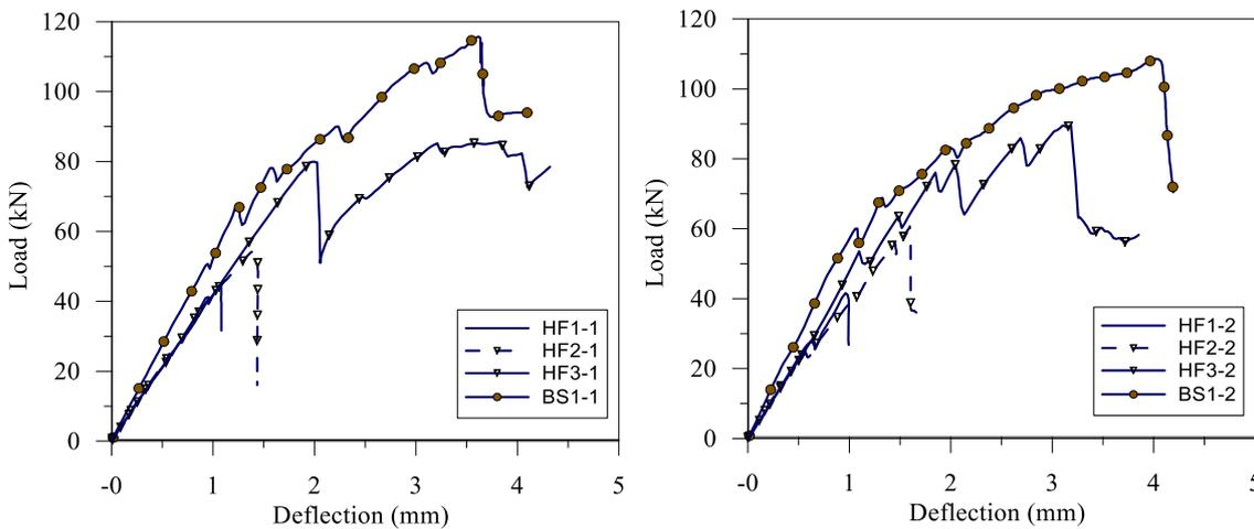
**Figure 6.** Load-deflection curves of eight short beams in 1<sup>st</sup> group
