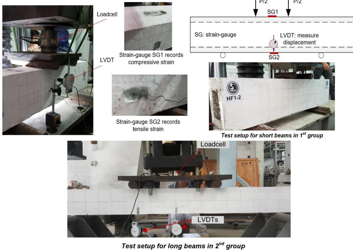
**Figure 5.** Test setup for short beams and long beams
