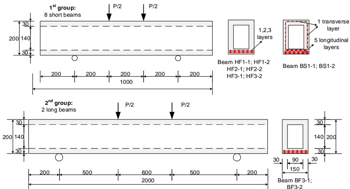
*Figure 2. Details of test beams in two groups*
