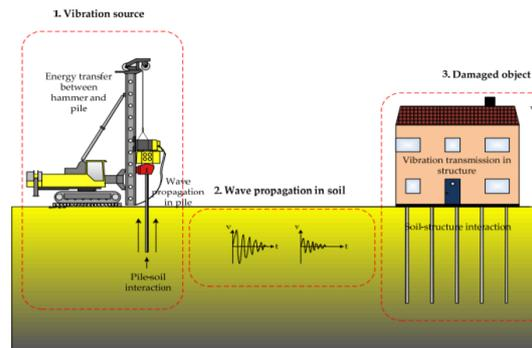
**Figure 9.** Vibration propagation process due to piling [1]
