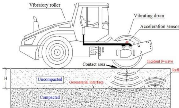
**Figure 8.** Principal components of a roller compactor with smooth drum [14]
