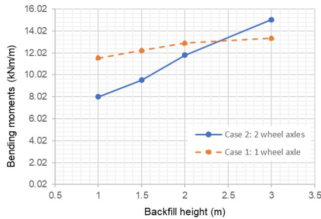
*Figure 12. Relationship between bending moments and thickness of backfill*
