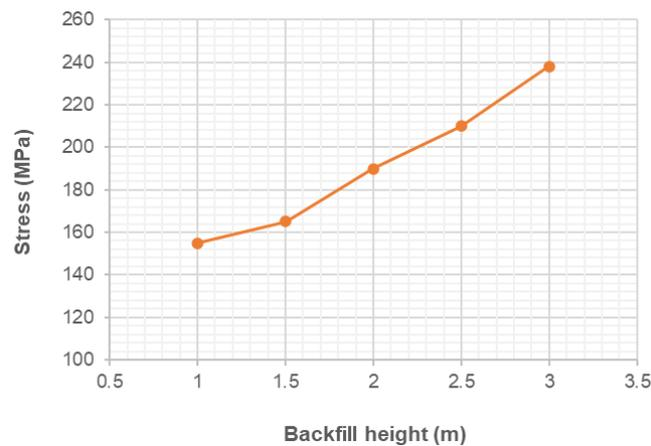
Figure 14. Relationship between stress and thickness of backfill
