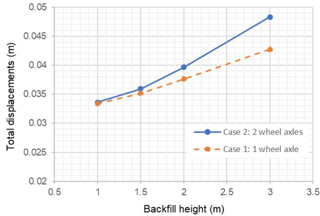
*Figure 11. Relationship between total displacement and thickness of backfill*
