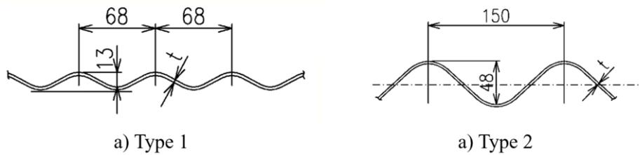
**Figure 7.** Dimensions of two types of corrugated steel pipes
