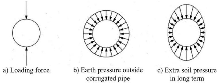
**Figure 5.** *The operation principle of corrugated pipes*
