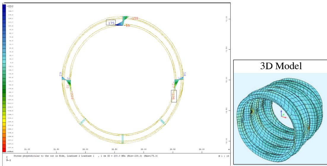
Figure 13. 3D model and the result of stress with backfill 3.0m
