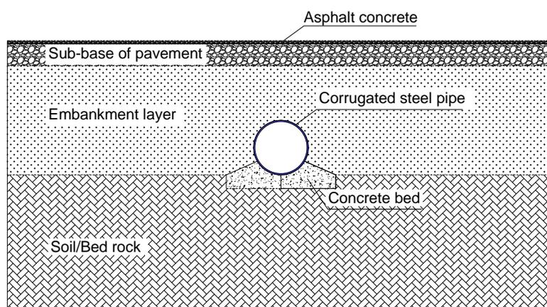
Figure 9. Example of corrugated steel culvert
