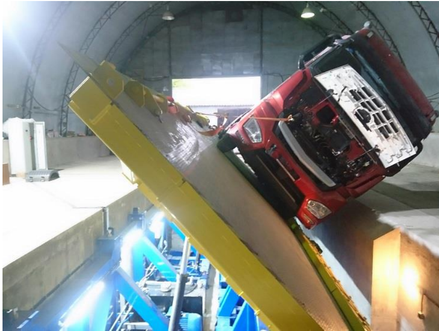
Fig. 2. Experimental determination of the transverse coordinate of the vehicle center of gravity
