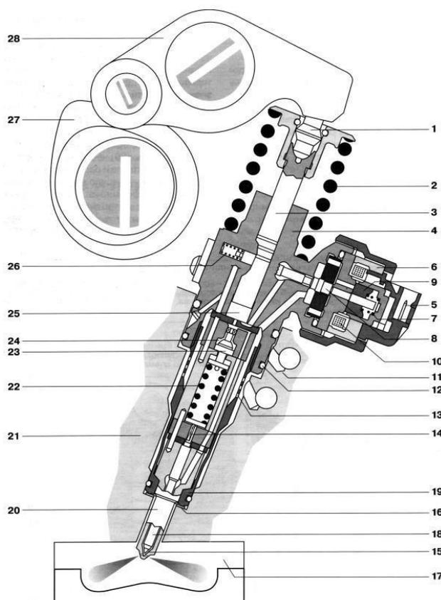
**Fig. 1.** Cummins injector for diesel engine
