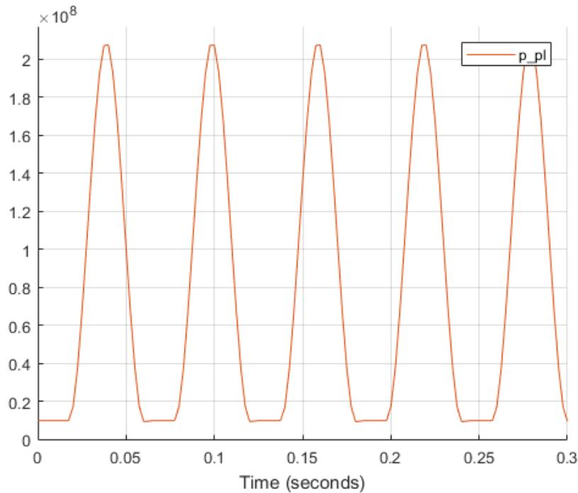
**Fig. 9.** Pressure in the plunger's chamber
