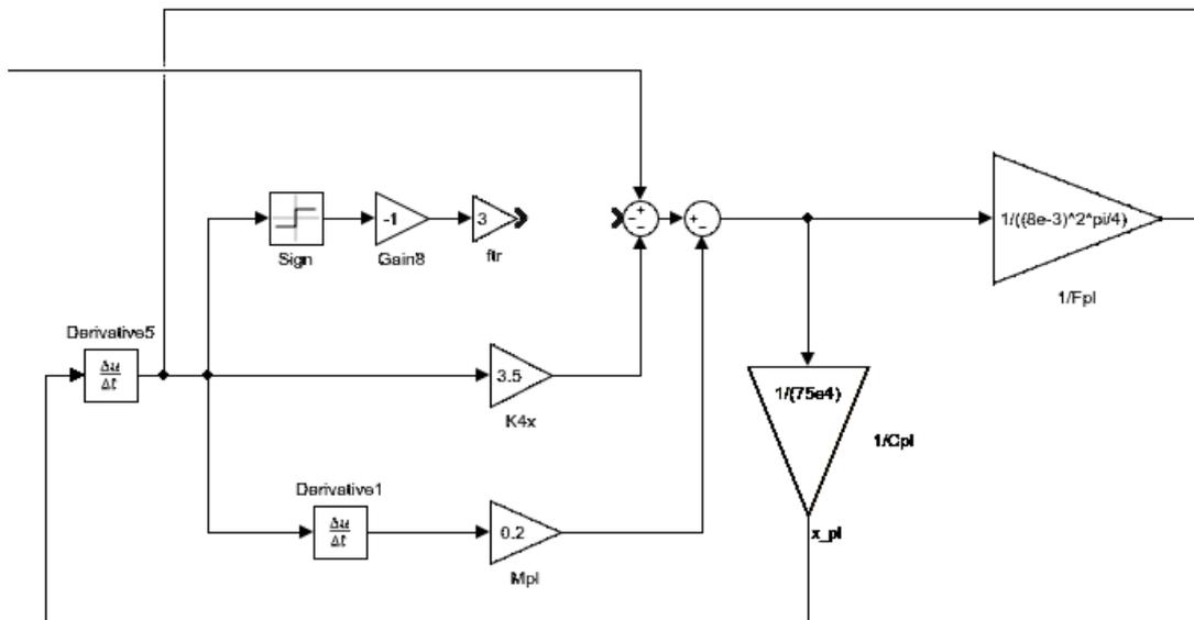
**Fig. 8.** Block diagram for calculating the movement of the plunger
