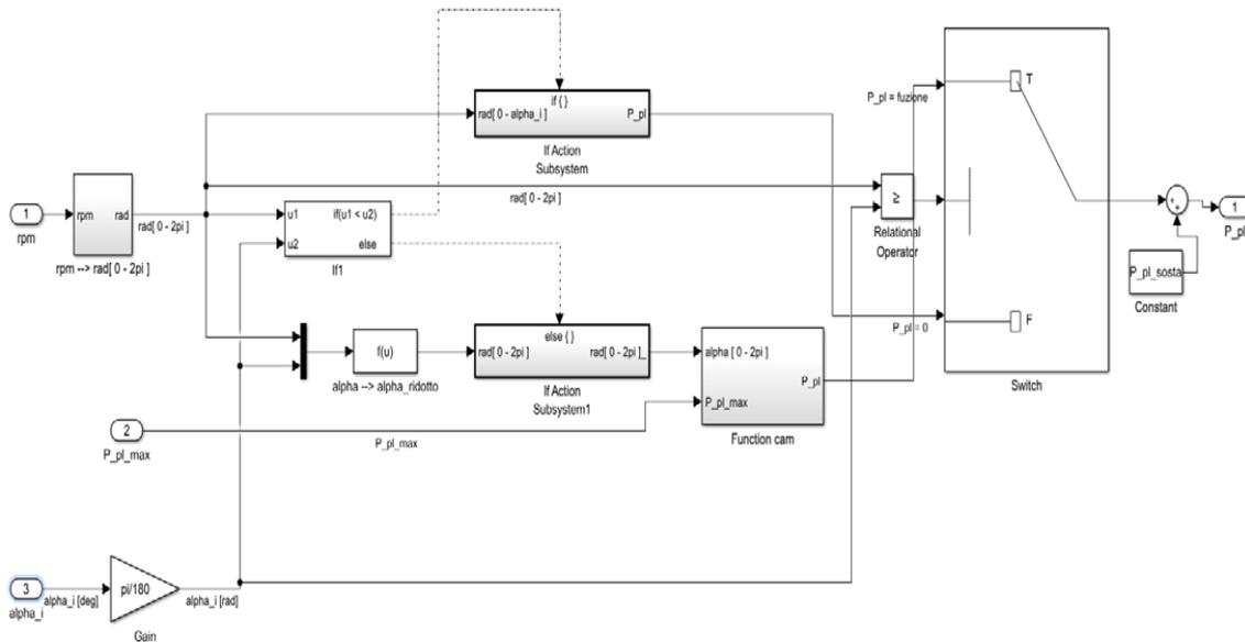
**Fig. 6. Block in which is calculated the cam force**
