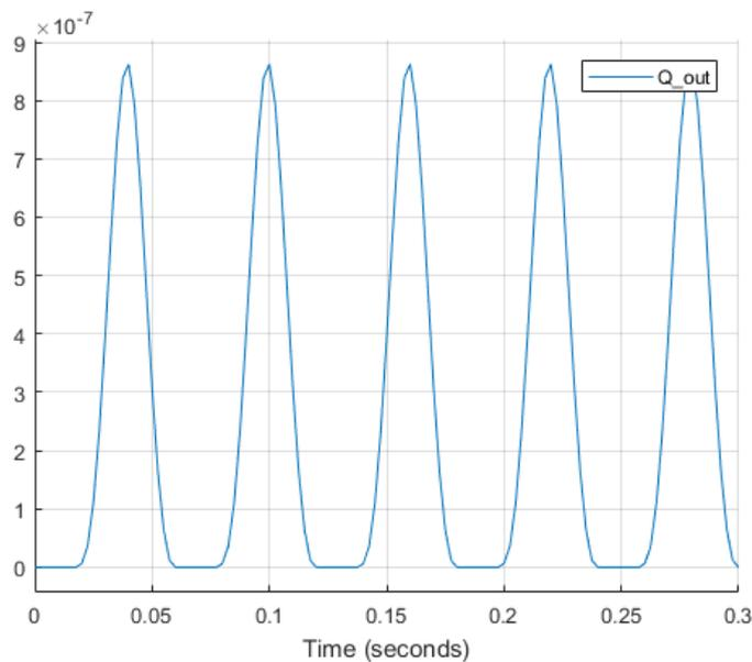
**Fig. 11.** Flow rate out of the injector
