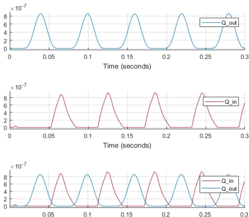
**Fig. 13.** Comparison between the flow rate which enters ( $Q_{in}$ ) and exits ( $Q_{out}$ ) the plunger chamber
