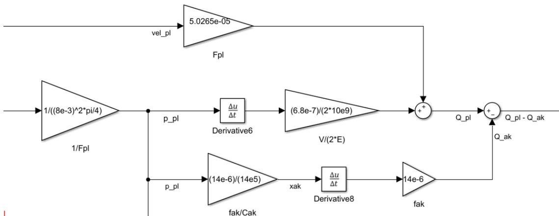
**Fig. 10.** Block in which is calculated the flow rate out of the injector
