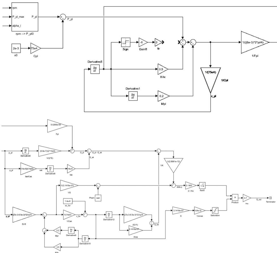
**Fig. 4.** Injector pump block in Simulink
