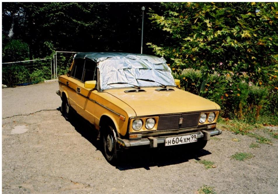
*Fig. 1. Temperature experiments when shielding the roof, the windscreen and rear windows*
