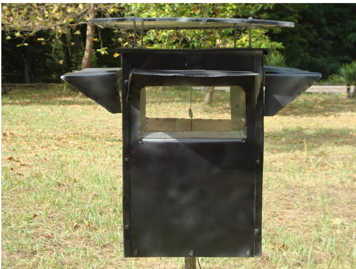
*Fig. 2. The layout of the cabin with the ability to rotate 360° relative to the sun and the ability to change the design of the thermal protection*
